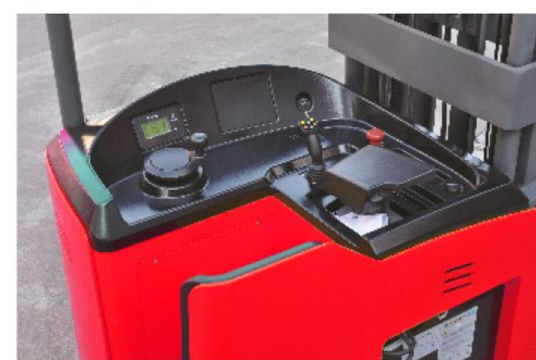
Curtis controller and display 36volt CURTIS AC control system, smaller electric current to ensure the reliability of the battery system. Multi-function display for battery status, hour meter, fault code, slow running state, etc.
