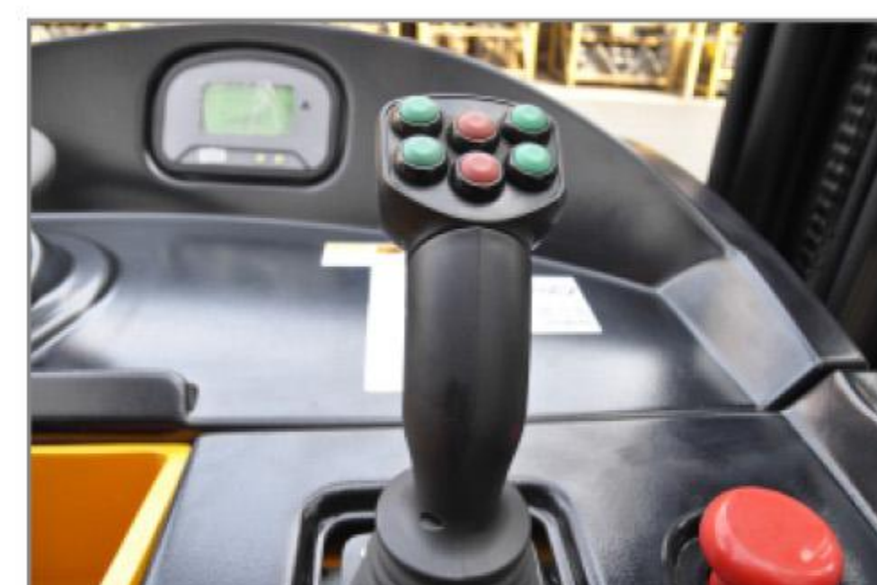
Control handle with integrated thumb stick, allows smooth operation of (1) Travel, (2) Lift/low, (3) controls Tilt and Fork Reach.
